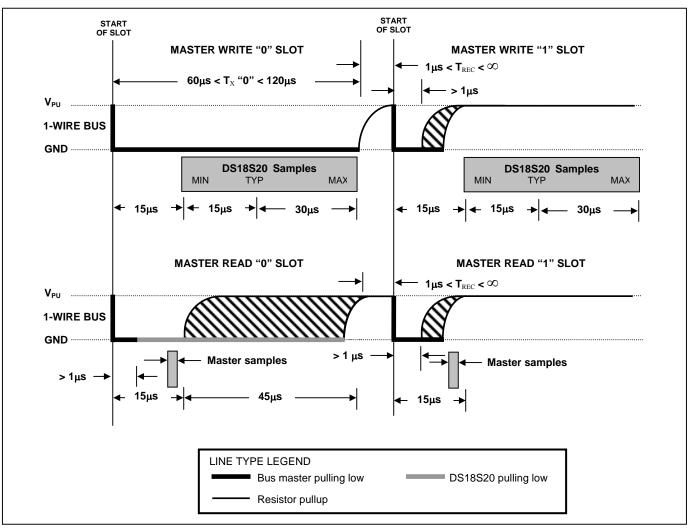
Figure 11. Read/Write Time Slot Timing Diagram
