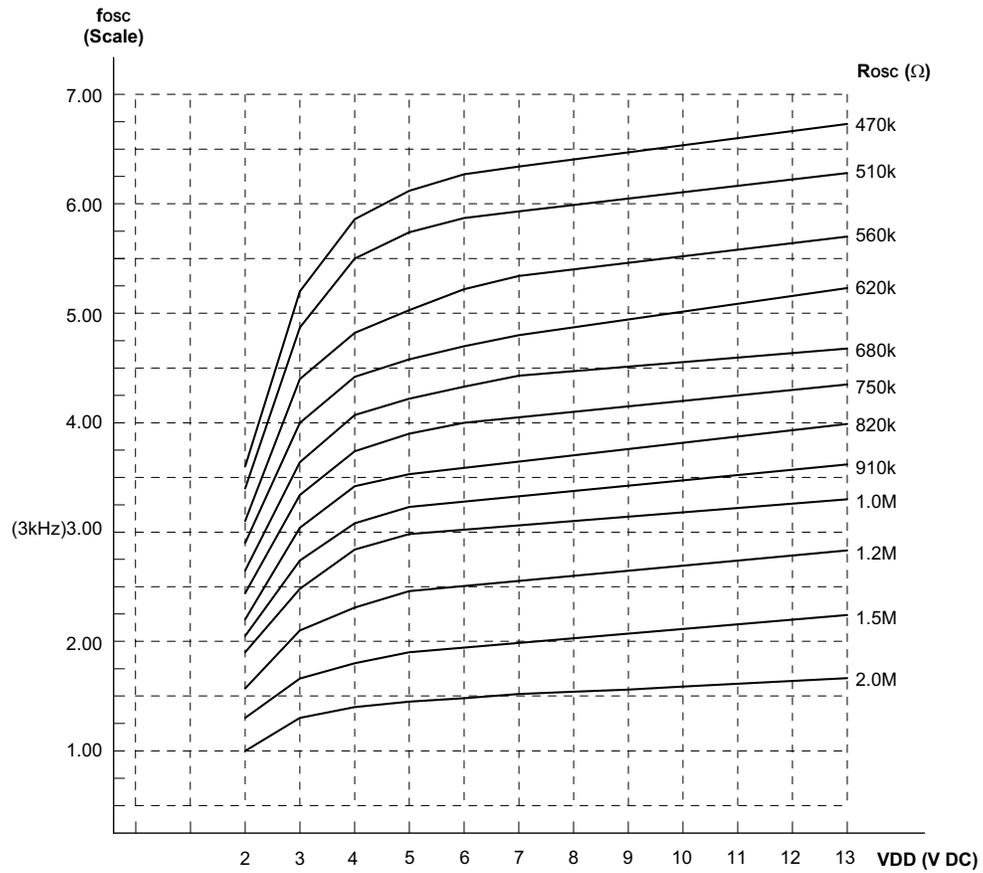
The recommended oscillator frequency is  $f_{OSCD}(\text{decoder}) \cong 50 f_{OSCE}(\text{HT12E encoder})$
