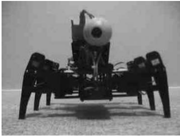
Fig. 1. MKIII hexapod mobile robot.
