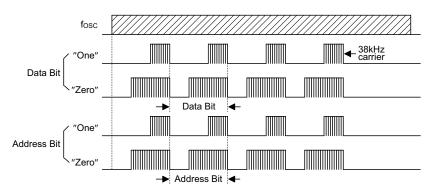
Address/Data bit waveform for the HT12A
