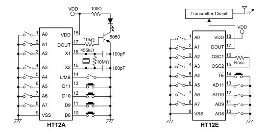
Notes: Typical infrared diode: EL-1L2 (KODENSHI CORP.) Typical RF transmitter: JR-220 (JUWA CORP.)
